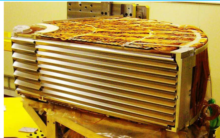
EMEC module construction ~1/4 of wheel assembled
