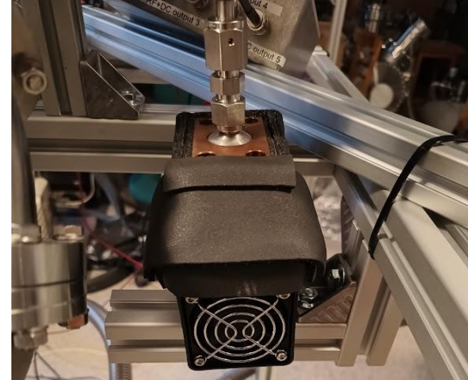
Thermal shielding for the reservoir designed and built by Adam Linek (the driver not presented in the picture)
