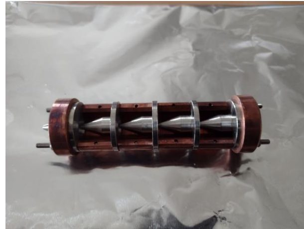
Thermal shielding for the reservoir designed and built by Adam Linek (the driver not presented in the picture)
