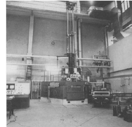
Fig. 4. Electron-beam melting furnace: 450 kW Leybold-Heraeus ESP 100/450.
