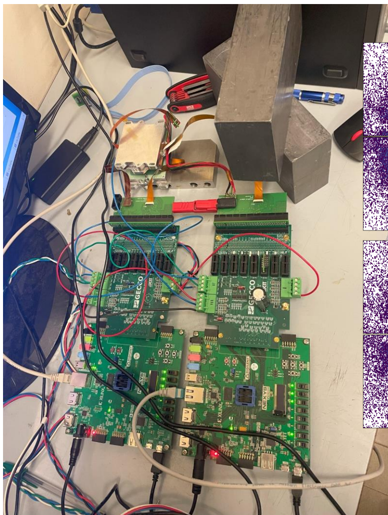
Two modules taking data with a 90Sr source Visible are the shadows of the data connectors
