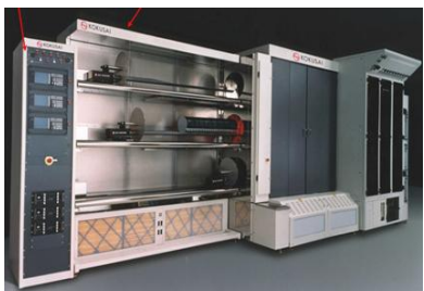
Oxygen/polycrystalline/annealing horizontal furnace tube/low stress silicon nitride LPCVD equipment
