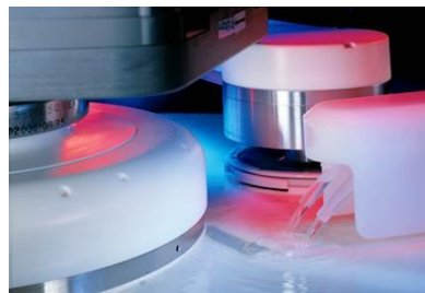
Chemical mechanical planarization CMP equipment
