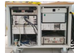
Stretched wire system SSW6, magnetic axis measurements FAIR Super-FRS multiports. Courtesy P.Kosek
