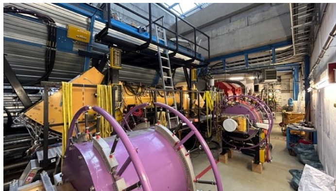
ESR electron cooler during Dec 2023 reassembly
