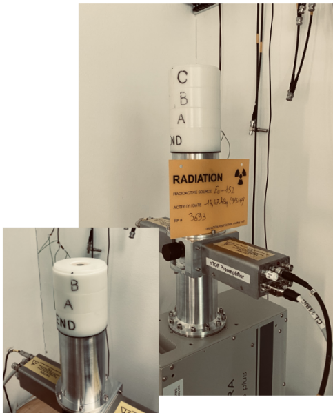
Fig. 9 The HPGe used for the induced activity measurements of this study. Different polyethylene spacers can also be seen.
