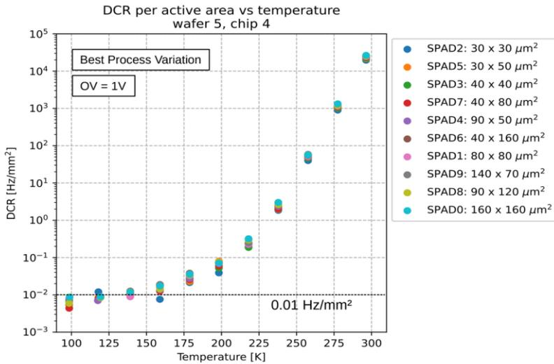
• DCR is <0.01 Hz/mm<sup>2</sup> @ 100K and 0.02 Hz/mm<sup>2</sup> @ LXe
