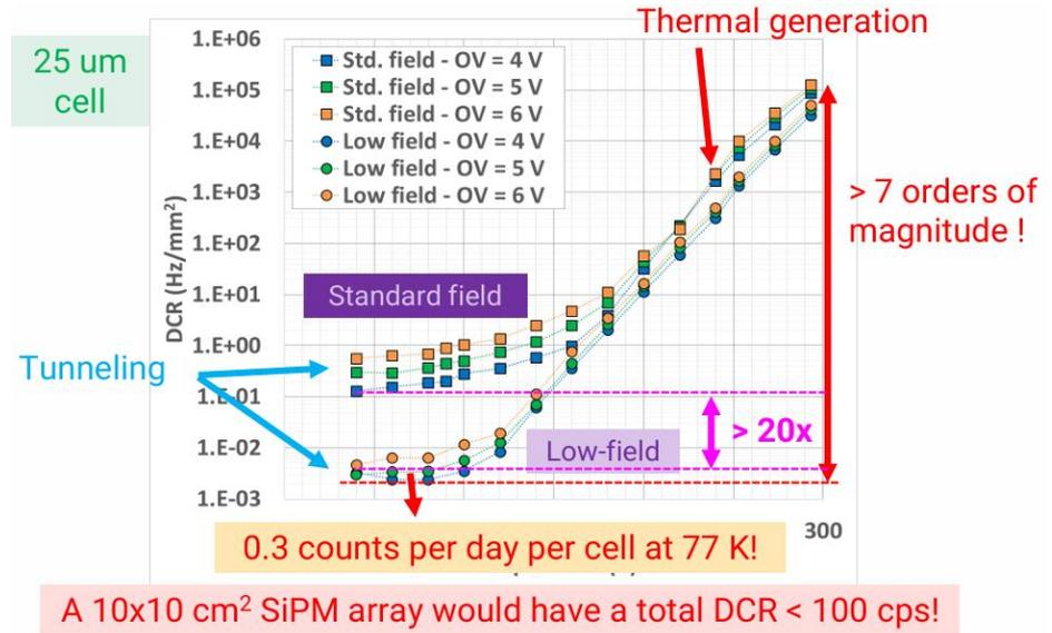
Reduction of Dark Count Rate at cryogenic temperature thanks to electric field engineering in FBK SiPMs.
