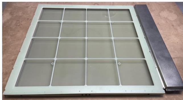
SiPMs-Based Photodetection Unit
