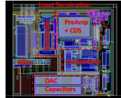
10b, 100KSPS in-pixel ADC ( $\sim 30 \times 30 \mu\text{m}$ )
