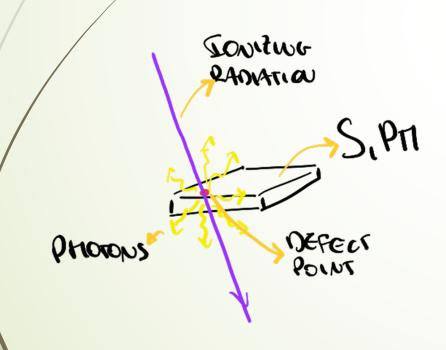
we can imagine a defect area in the sensor that, once excited by external ionizing radiation, releases photons with a typical lifetime of the order of ms that can then be detected by the SiPM itself producing thus the burst.
