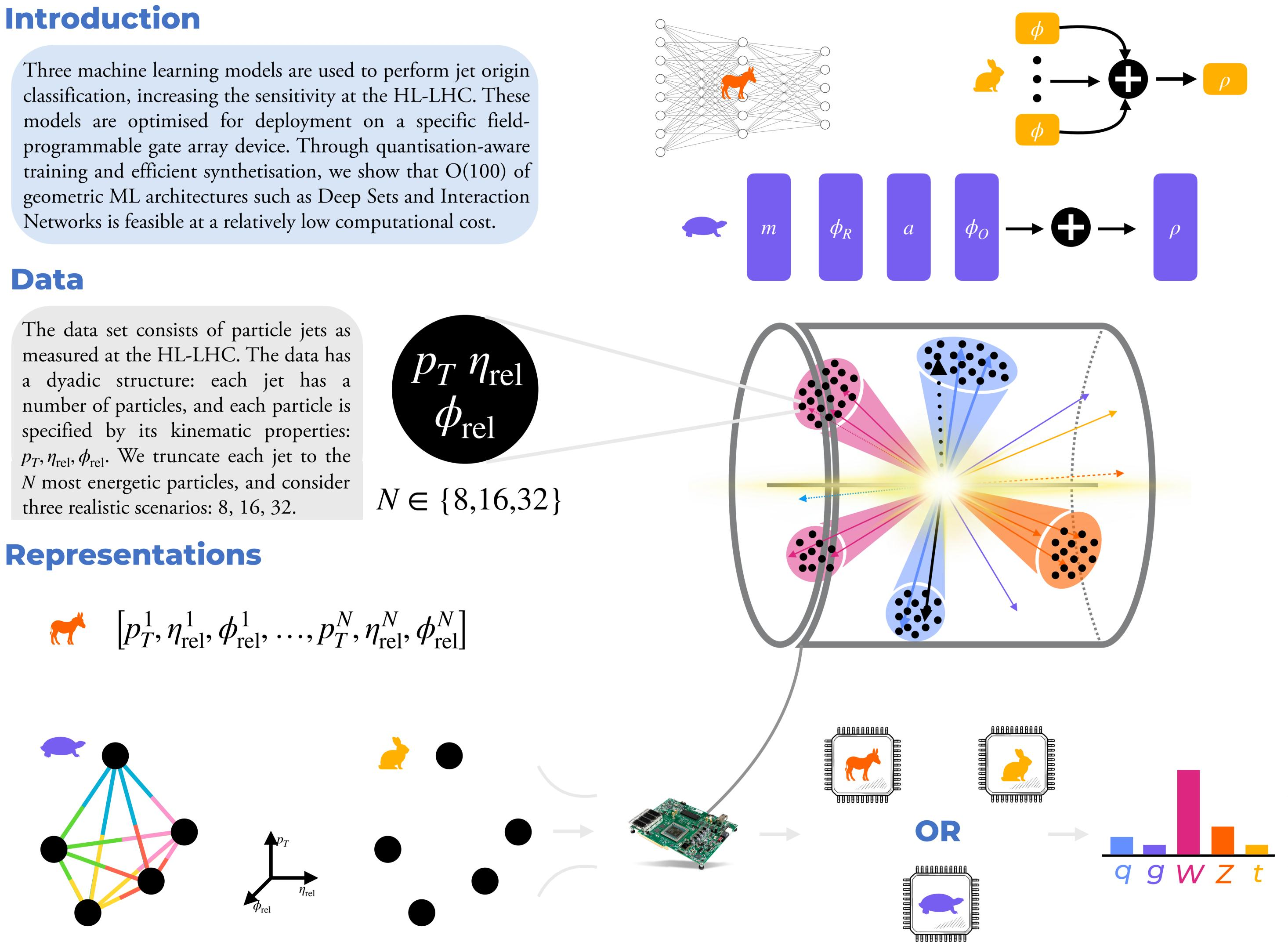
The data can be represented in  $p_T$ ,  $\eta_{rel}$ ,  $\phi_{rel}$  space in three ways: tabular, set, and fully-connected graph. These representations correspond to different deep learning architectures: multi-layer perceptron, deep sets, and interaction network, respectively. There exist other representations of the data; however, these three are arguably the simplest.
