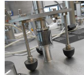
Damping bellow connecting liquefier, top of the cryostat
