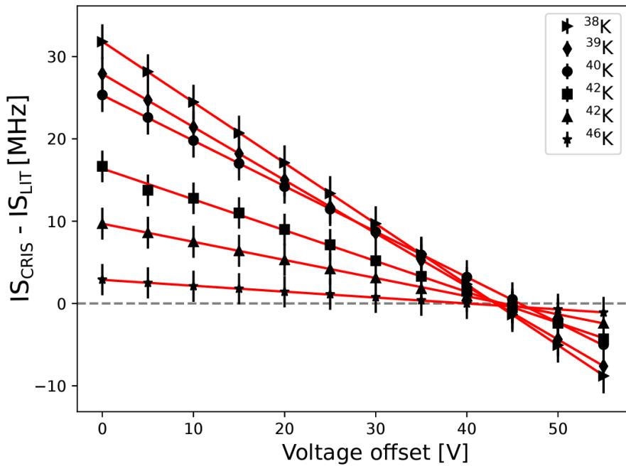
Voltage calibration necessary over long range of isotopes
