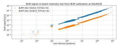
500kW -> 5.8e11 protons/s 6 orders of magnitude bewlo max loss allowed for RS09
