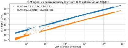
In all cases signal in new BLMs visible from losses around 3e5 protons/s
