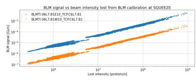
500kW -> 5.8e11 protons/s Good sensitivity around 6 orders of magnitude below max loss allowed for RS09
