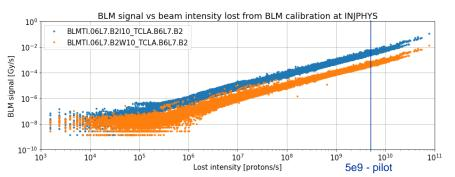
In all cases signal in new BLMs visible from at least losses around 1e6 protons/s
