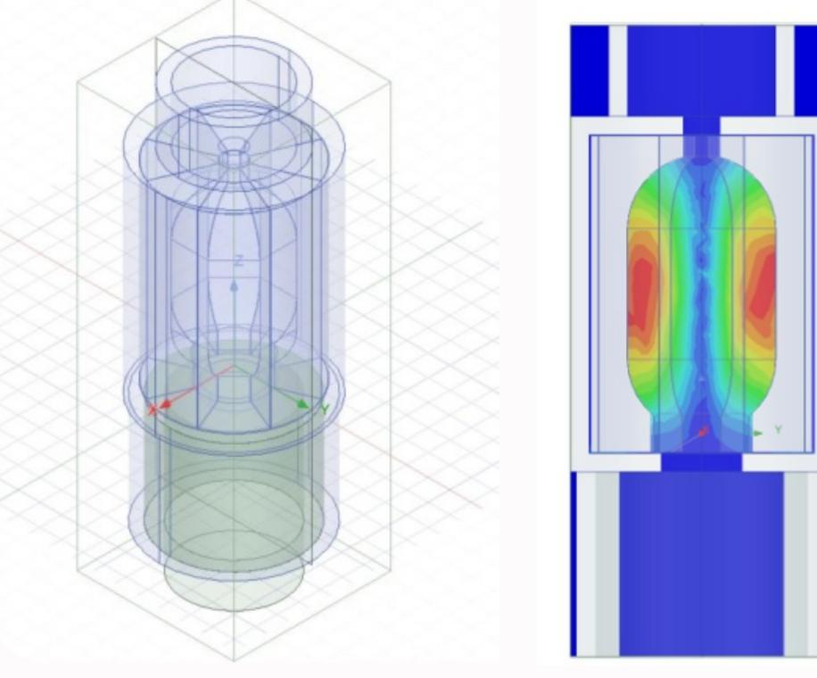
Octagonal cavity exciting the TM010 mode was designed. This allows currents to run longitudinally. Cavity is formed from 8 facets, each of which can have High Temperature Superconductor (HTS) tapes laid along their inner surface.
