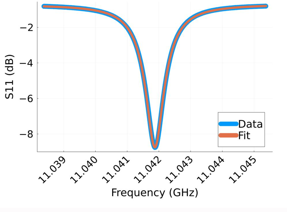
HFSS simulation shows similar results, but different frequency due to radial shifts in assembly.
