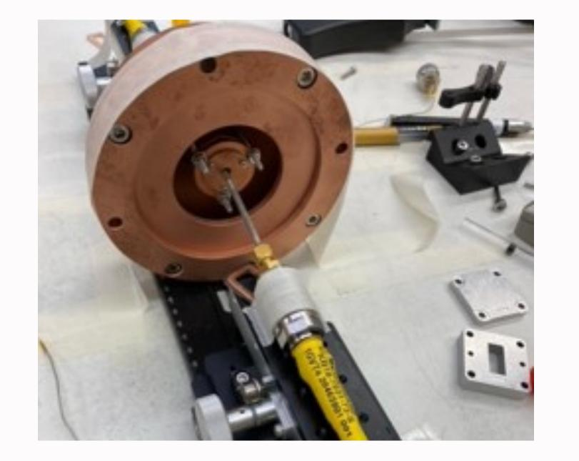
S21 measurements with coaxial probes verified the singular mode within the bandwidth of interest.
