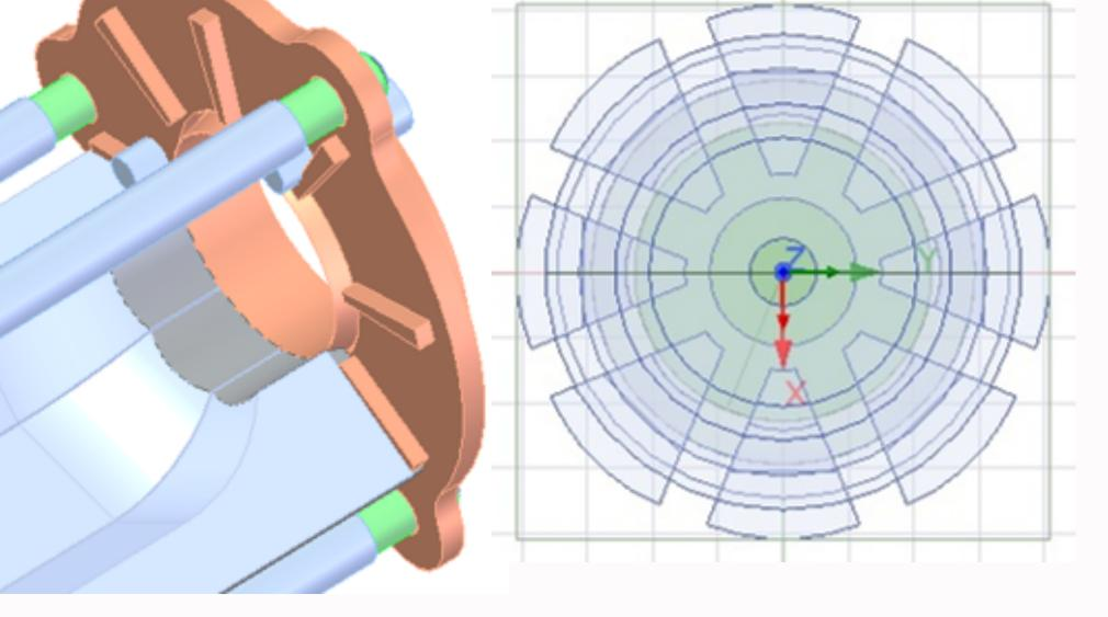
Tuning frequency and coupling is done by radially shifting the facets. This shift is handled by small wedges on the end caps, which align the facets as well. Detuning is about 100 MHz/mm.
