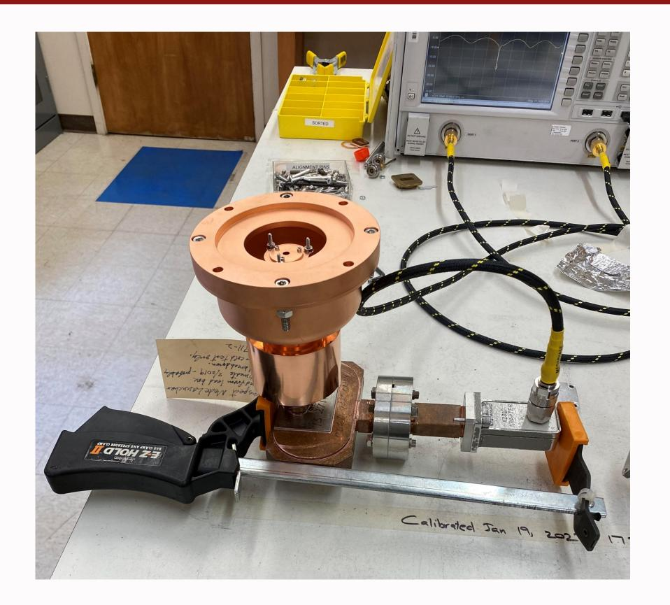
Measurements were done with a TM01 mode launcher clamped to hemispherical vessel.
