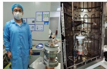
Degassing furnace evacuation
