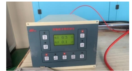
Vacuum condition of the prototype upon arrival
