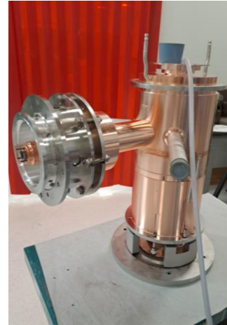
penultimate and last cavities + window
