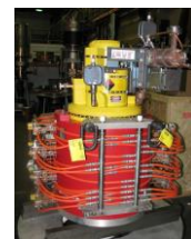
2011 – 50 MW 12 GHz Klystron, CERN
