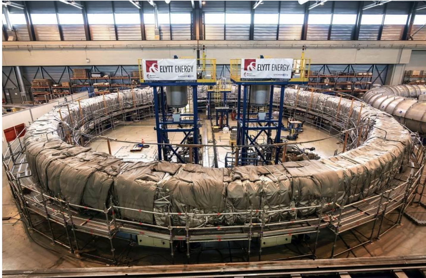
Impregnation of an ITER PF coil performed by ELYTT Energy (our largest magnet)
