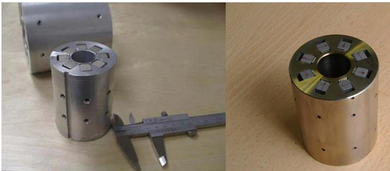
Hallbach quadrupoles for Linac4 at CERN (our smallest magnet)
