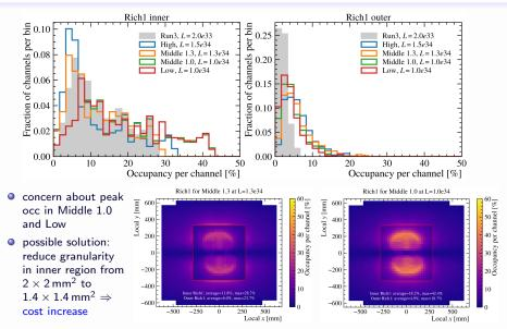
$\Rightarrow$  study of different geometries to distribute photons on the focal plane
