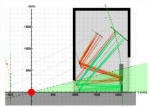
In both cases the study of the space available in the cavern is crucial: larger radius of curvature implies moving the photon detector panels further away from the beampipe
