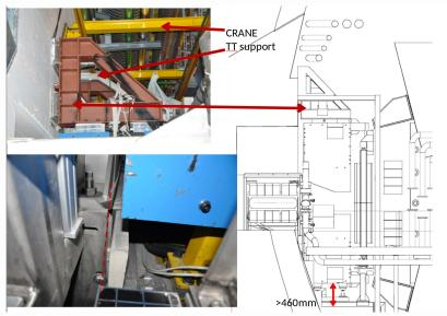
Very tight constraints both above and below RICH1: study of the removal of the magnetic shielding to gain more space for cryo and focal length
