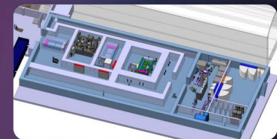
BDF target complex building with service cell
