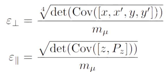
Calculate single-particle scattered emittance
