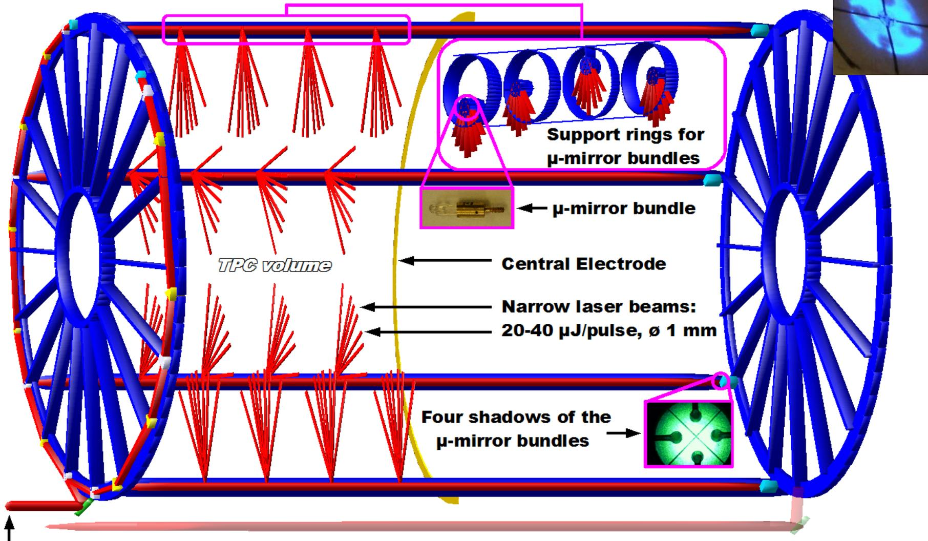
Wide laser beams: 266 nm,
