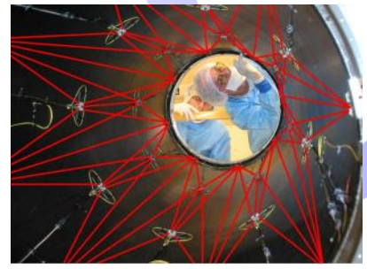
Figure 1: Grid line Interferometer layout on SCT Barrel flanges.
