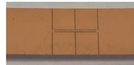
Laser cut bridge on REBCO at KIT
