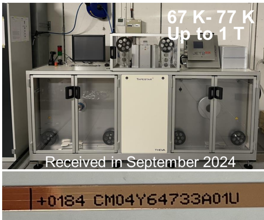
Tape marking and width/thickness measurement
