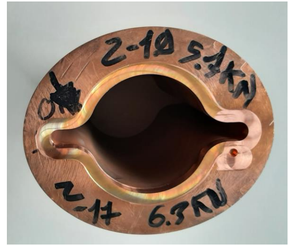
Stir welded flange after local remachining
