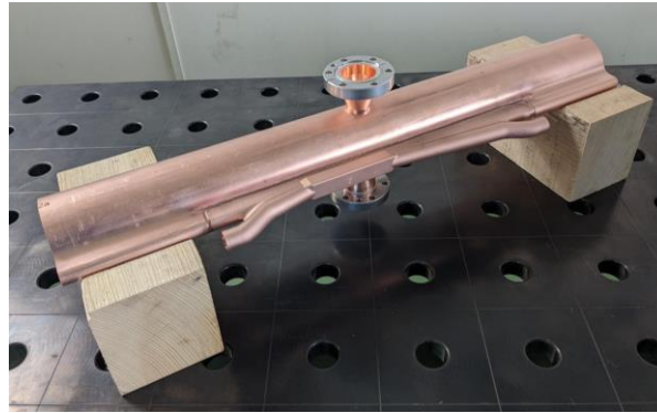
FCC-ee vacuum chamber prototype and leak test preparation
