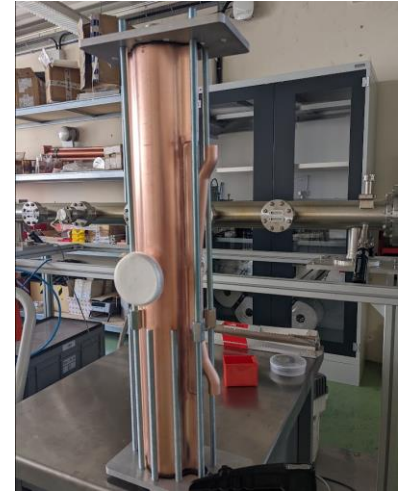
FCC-ee vacuum chamber prototype and leak test preparation
