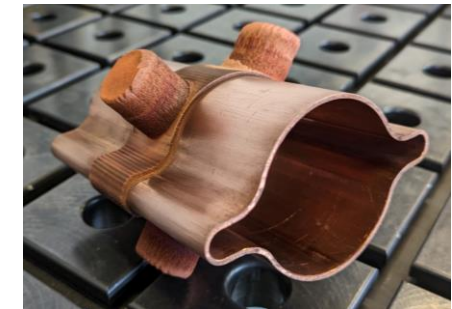
Test of cold sprayed bosses on a plate and chamber prototype
