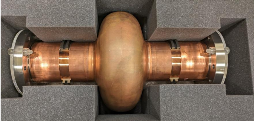
1.3 GHz hydroforming (KEK Collaboration)
