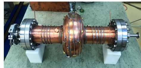
Radiofrequency (1.3 GHz) Cu cavity with soldered capillary
