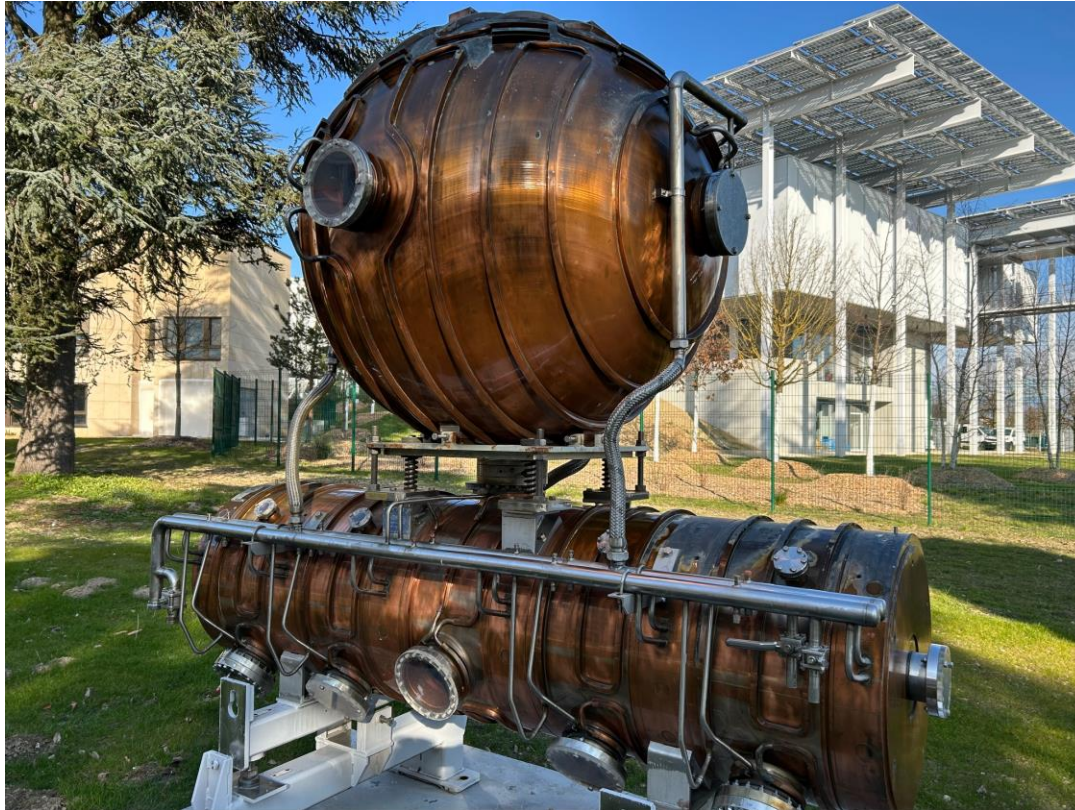
Cu cavity with water cooling circuits
