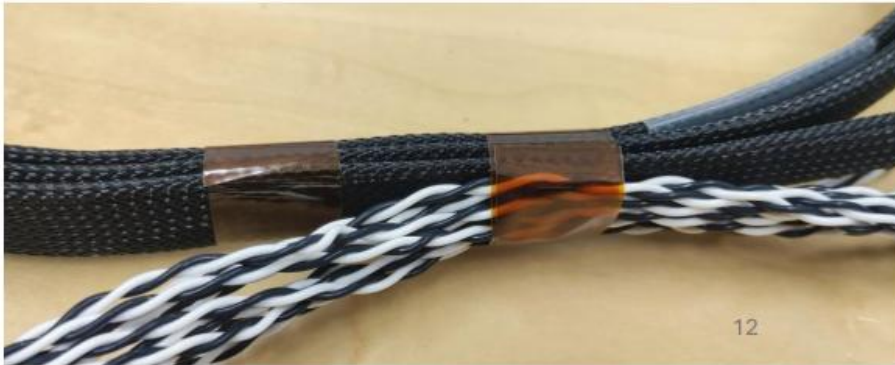
One option of 3 data cables + power cable for the front-end board of cold electronics.
