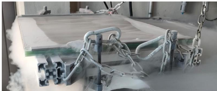
One setup of cold test: clamped to the frame
