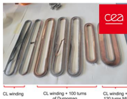
CEA process development for metal-insulated racetrack coils.
