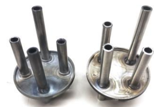
Fig. Welding test (left) mock-up of tantalum and (right) stainless steel used for training [A]
