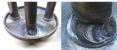
Fig. Welding test for the Ta-Ta joint on the HIPing capsule (left) mock-up and (right) zoom of the resulting joint [A]
