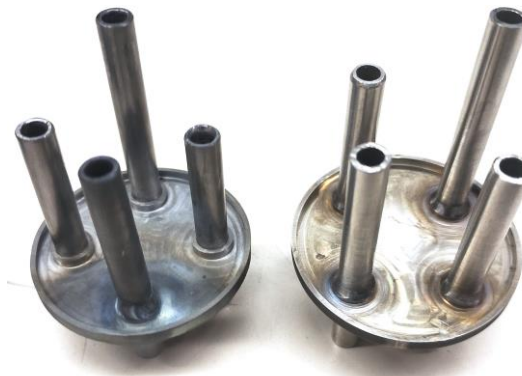
Fig. Welding test (left) mock-up of tantalum and (right) stainless steel used for training [A]
