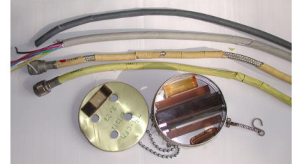
Radiated equipment in LEP
