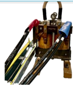
0.4 mH Inductor added for the 200 A circuit
