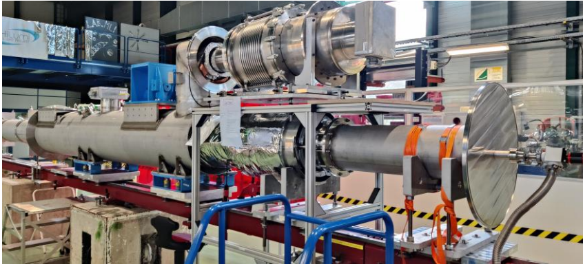
Leak test in progress on the DCM
