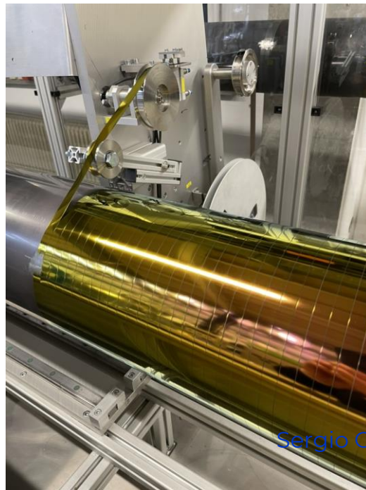
Roll to roll coater for HTS tapes
