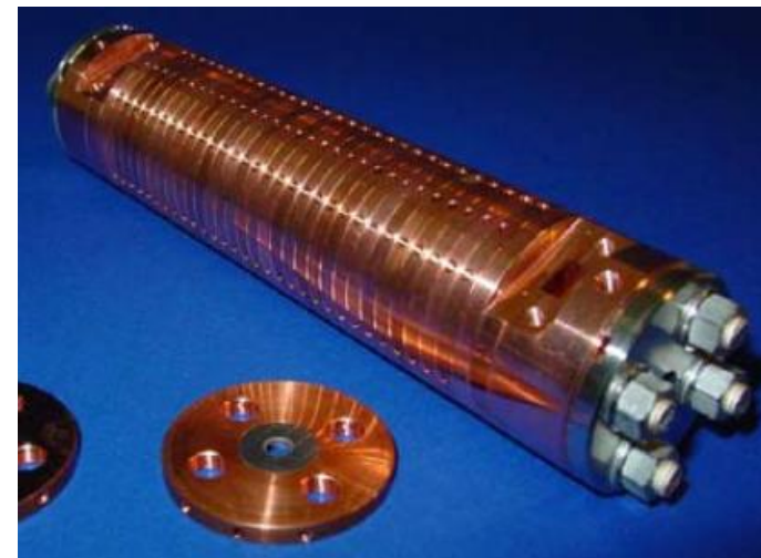
NC copper, Q_0 \approx 10^4 , 100 MV/m, pulsed
