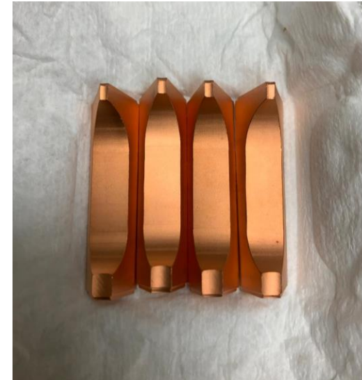
SLAC Segmented cavity for RF pulse compressor
