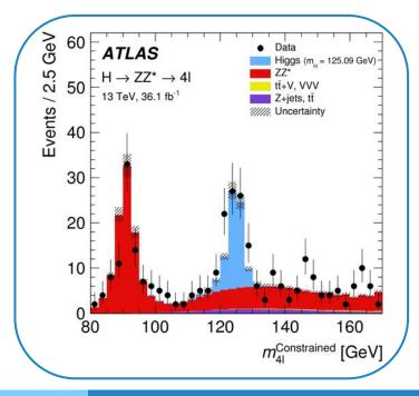
Here we see an example of a Higgs boson analysis which plots the the combined mass of four particles (leptons)
