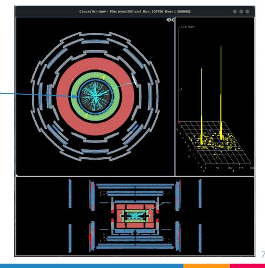
• This is the <u>main detector window</u>, which shows the main sub-detectors and the various tracks and energy deposits.
