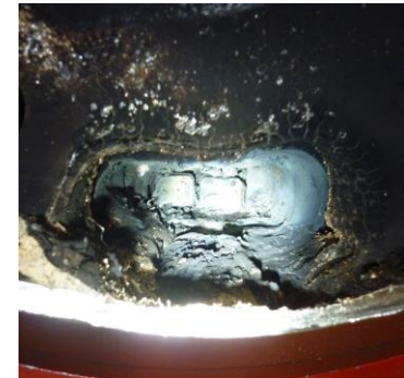
Pictures of a short in MB1109 (C23R3). 226m away from the incident started in Sector 3-4 in 2008
