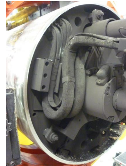
Pictures of a short in MB1109 (C23R3). 226m away from the incident started in Sector 3-4 in 2008
