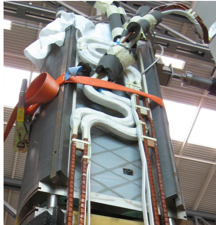
LHC SSS QF and QD busses integration inside the yoke
