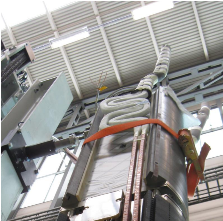
LHC SSS MB busses integration inside the yoke
