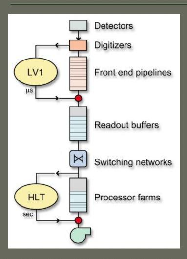
Level-1 Trigger (L1T) –Hardware – 40 MHz to100 kHz
