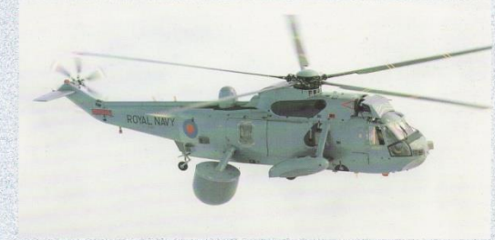
A Royal Navy Sea King helicopter fitted with the airborne early warning version of the Searchwater radar (Photograph by courtesy of Thorn EMI Electronics Limited).
