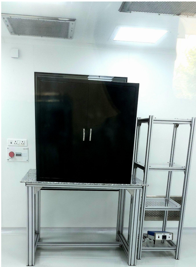
Probe station with dark box in clean room (class 1000)
