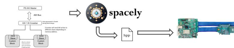
(1) Build a firmware design in Vivado by connecting pre-made AXI blocks (no RTL experience required unless you need custom blocks)
