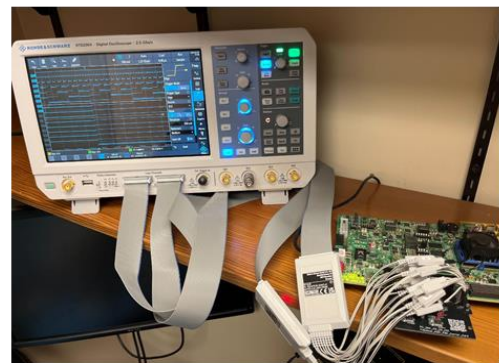
Outputs from eFPGA (16b counter) probed with oscilloscope
