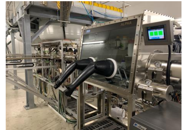
A Photocathode Preparation Facility (PPF)
