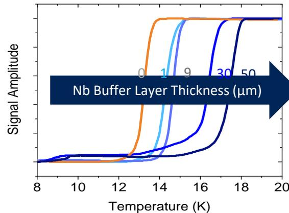
$T_c = 17.33 \pm 0.25$  K on Cu + 50  $\mu m$  Nb Buffer Layer at  $T_{dep} = 600$  °C
