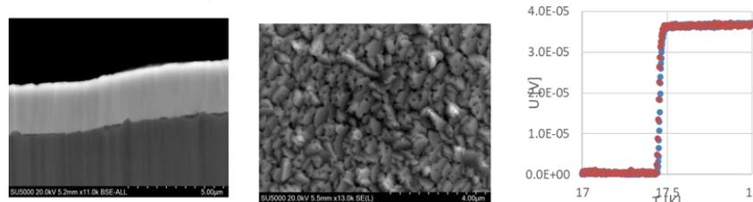
100 W HiPIMS  $\text{Nb}_3\text{Sn}$  on 50 and 100 mm diamond turned Cu
