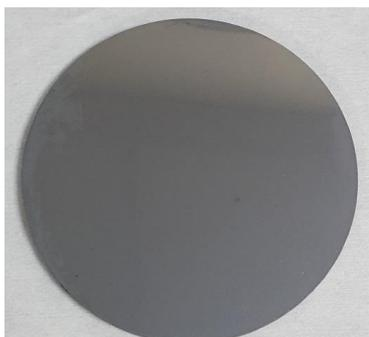
100 W DC  $\text{Nb}_3\text{Sn}$  on 50 and 100 mm diamond turned Cu
