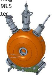
Hadron Storage Ring - 197 MHz bunch compression cavity IR04
