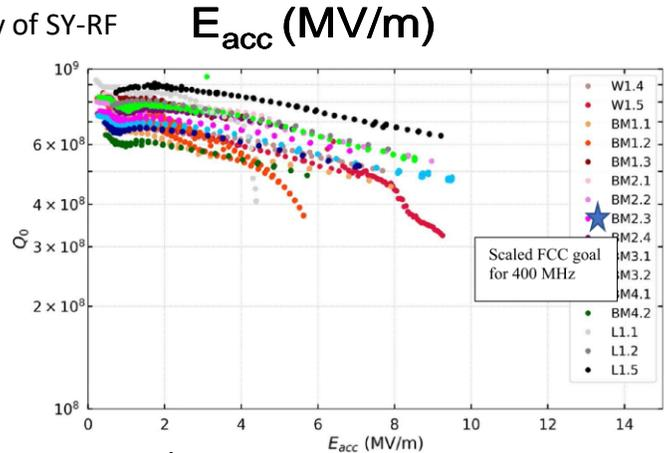
1.3 GHz HiPIMS Nb/Cu cavities performance at 4.2 K
