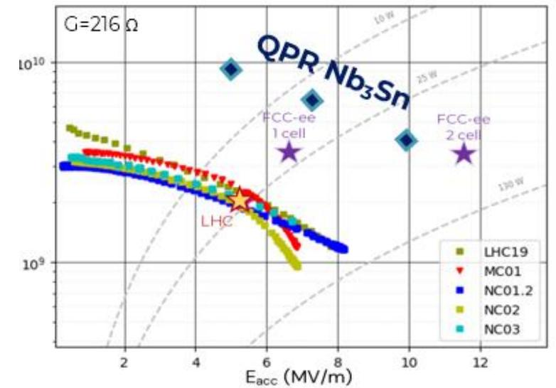
$Nb_3Sn$  on bulk Nb to validate coating performances on 1.3 GHz Elliptical Cavities (2025)
