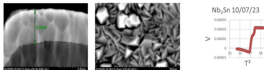
50 W DC  $\text{Nb}_3\text{Sn}$  on 50 and 100 mm diamond turned Cu
