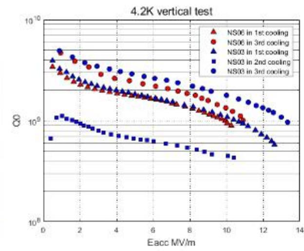
Vertical tests at different cooling rate
