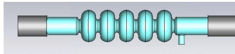
5-cell 591MHz cavity scaled from e-RHIC ERL 650MHz
