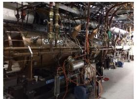
Hadron Storage Ring – 24.6 MHz acceleration cavity IR04
