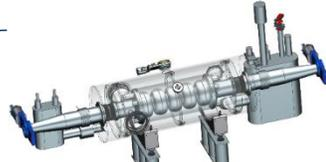
Hadron Cooling - 591 MHz acceleration cavity
