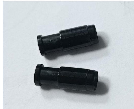
End-plug and spacer mechanical precision – 5 μm (the same as the one of the inned straw diameter)
