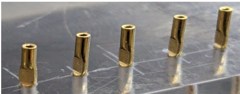
End-plug and spacer mechanical precision – 5 μm (the same as the one of the inned straw diameter)
