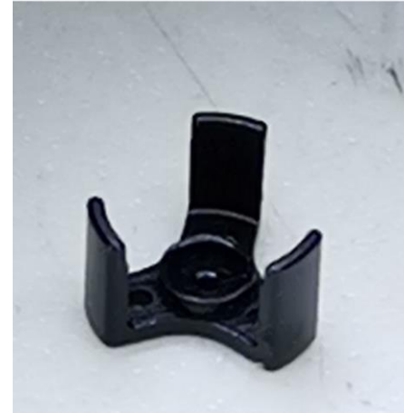
End-plug and spacer mechanical precision – 5 μm (the same as the one of the inned straw diameter)
