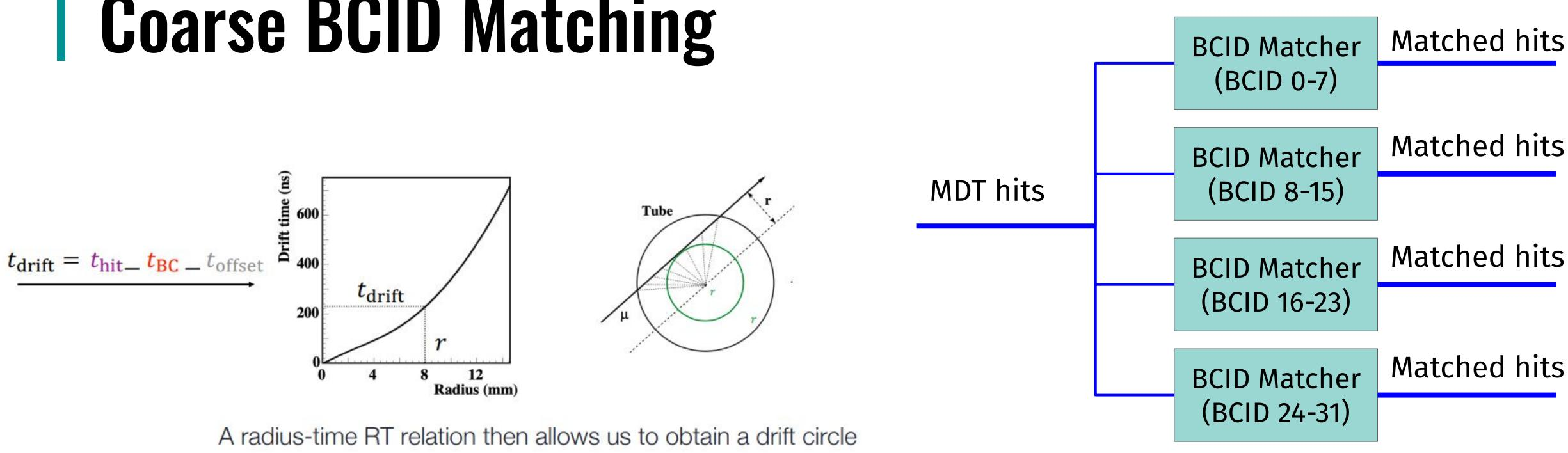
• Each drift-tube hit is compatible with 32 possible bunch crossings • Maximum drift time 800 ns, FCC bunch crossing period 25 ns • Number of BCID matcher blocks at FCC-hh will depend on BC spacing and actual tube radius • If 7.5mm radius tubes, only one block is required
