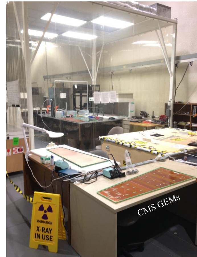
FIT Clean Room: assembly of CMS GE1/1 GE2/1 and ME0 GEMs
