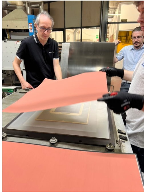
Pressing stack preparation with layers of: copper, conformable layer (pacoflex), cushions, ...
