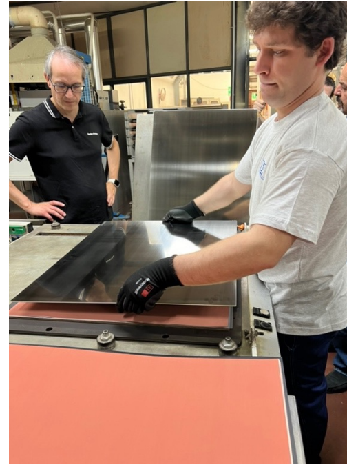
Pressing stack preparation with layers of: copper, conformable layer (pacoflex), cushions, ...
